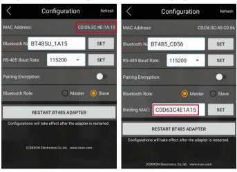
• There is only one BT485U Bluetooth slave role in wireless RS-485 network, while there can be up to 20 BT485 Bluetooth masters. Just add the masters to network one by one by repeating the Bluetooth master configuration step.
