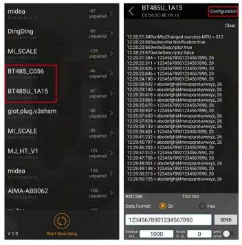
right corner will enter configuration interface. The first access to the interface requires password verification, and the default access password is 5 letters: "irxon".
